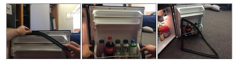
• After all the screws are loose, the door seal should slide off fairly easy. Slowly remove the door seal with your hands by peeling it off the seal's shell.
