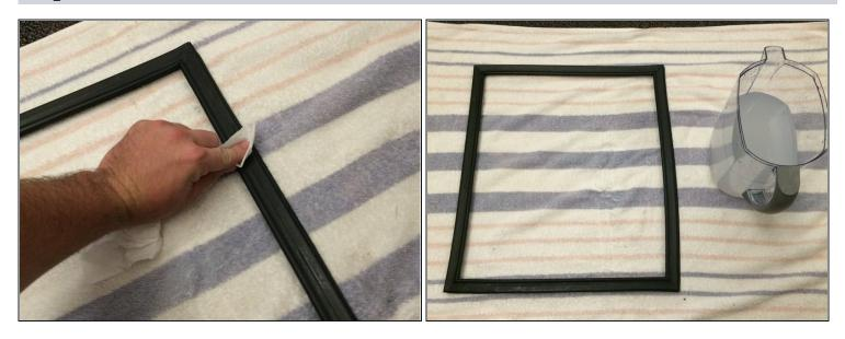
• On the side that connects to the refrigerator unit, apply a thin layer of silicon grease. This will improve functionality as well as prevent the seal from cracking in the future.
