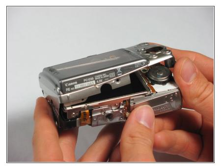
Slide the back casing (with the screen protector) off to reveal the LCD and back wiring.
