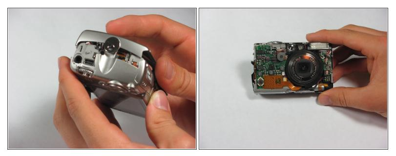
Gently pull the front cover straight out from the camera. This will expose the wiring on the front of the camera.
