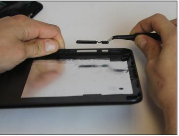
• Carefully place the bottom lid next to the screen case. The power/speaker buttons should be visible at the corner of the lid. Remove the buttons with the tweezers.
