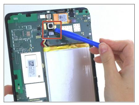
Use the plastic opening tool to disconnect the camera from the logic board, by prying it up.
