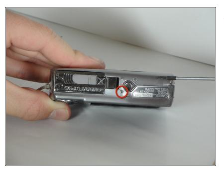
Remove one 2.25mm screw on the bottom.
