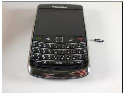
• Use your T5 Torx screwdriver to remove the two black 5.57mm Torx head screws underneath the keyboard.
