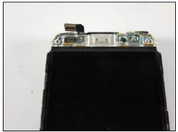
• Gently pry up the ribbon connector at the top of the phone with a plastic opening tool.
