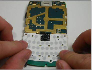
Align the new keyboard membrane with gold conduits and press down onto circuit board.
