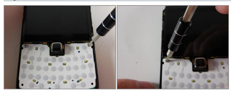
• Remove the two Torx head 4.13mm steel screws with your T5 Torx screwdriver.
