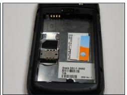
Slide the SIM card from underneath the holding bracket upward toward the battery connector pins.
