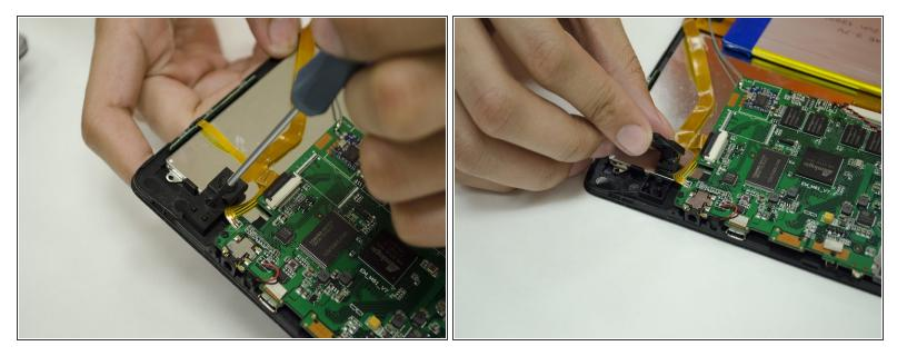
• Remove the #00 Screw holding down the Camera mount, then remove the Camera mount.
