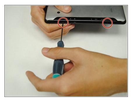
Remove the two Phillips #00 screws on the side of the tablet.
