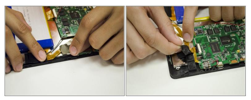
Slowly remove the two pieces of electrical tape holding down the Camera ribbon cable.
