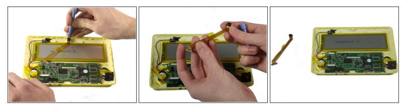
• Use a plastic opening tool to pry the camera out of its place.
