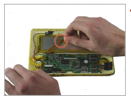
• Pull off the tape that holds the ribbon cable to the battery.
