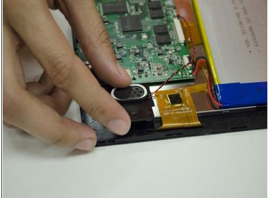
Remove the #00 screw on the Speaker mount and remove the Speaker mount.
