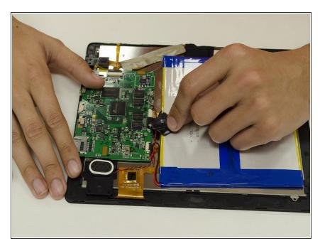
Slowly remove the electrical tape holding down the Speaker wires.
