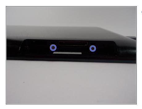
Remove the two screws using a PH #00 Phillips head screw driver.
