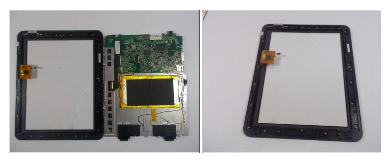
• Place the metal frame plate and components into the new plastic front panel.
