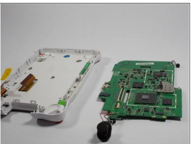
Lift motherboard to separate it the from the case shell.
