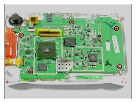
Use the Philips #00 screwdriver to remove the 5 screws from the motherboard
