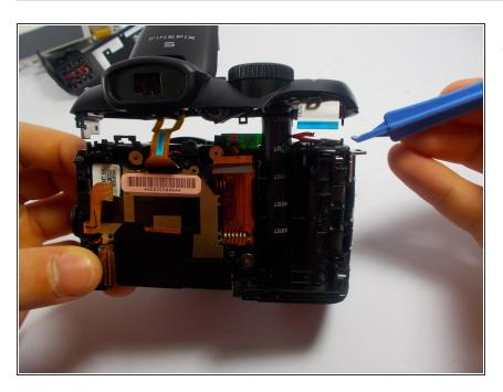
Pry the top of the camera off using the given tool
