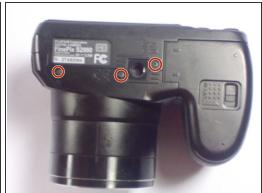
Use a PH0 screwdriver to remove four screws on the right side, three screws on the bottom, and four on the left side to take off the rear plate.
