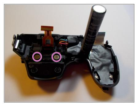
Remove two silver plated screw from under the top of the camera, under the flash.
