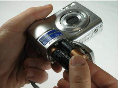
• Pull the batteries out of the device.
