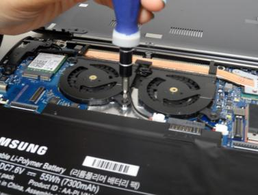
Using a Phillips head screwdriver, unscrew four 4.55 mm Phillips #000 screws that bind the fans.
