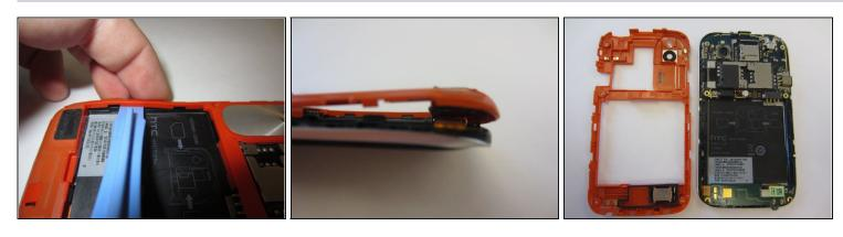
• Use an opening tool or a spudger to gently remove the rear frame.
