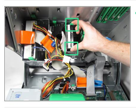
Pinch the two green tabs inwards to release the hard drive and lift it out.
