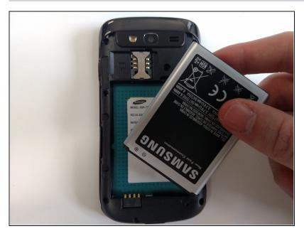
• Remove the battery from the device and set aside.
