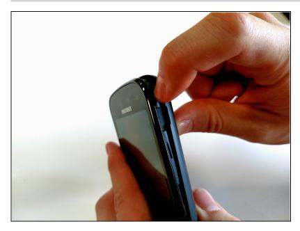
Start by removing the back plate to expose the battery by pulling the back and front plates apart.
