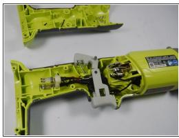
Now that the two halves are unscrewed, remove the top half
