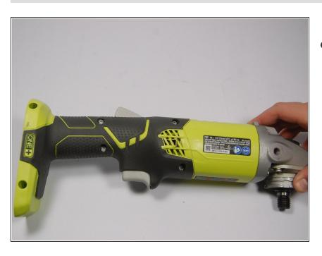
Lay grinder flat on its side so the screws are facing up
