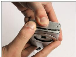
Pry apart the camera casing using the plastic opening tool tool provided. Once the casing has begun to separate pull the two sides apart with your hands.
