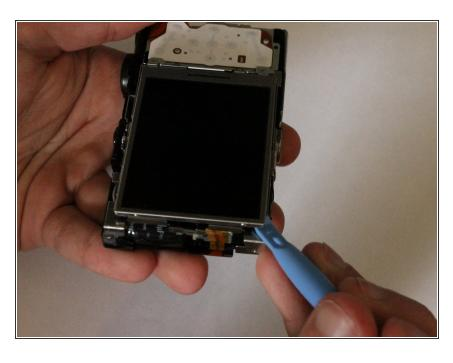
Pop the LCD display out of its frame using the plastic opening tool in order to get to the screws under the
