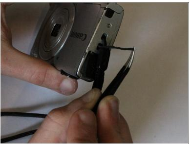
Remove the knot holding the wrist lanyard onto the camera
