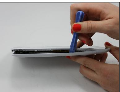
Use the plastic opening tool to assist in removing the back cover.
