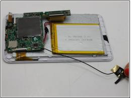
Remove the black and gold tab connecting the battery to the tablet's frame.
