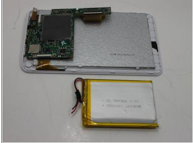
Remove the battery from the tablet.
