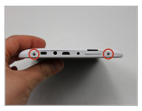
Remove the two 2.5mm screws using the Phillips #00 precision screwdriver.
