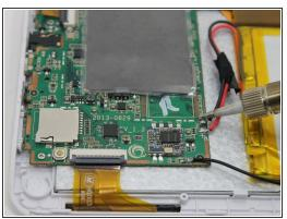
Install the new battery by soldering the three wires to the motherboard. For additional soldering
