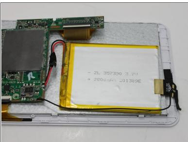
Remove any tape that might be holding the wires in place.
