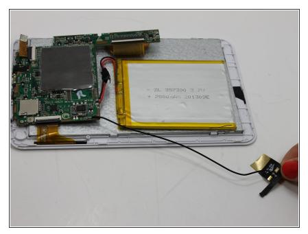
Remove the the one red and two black wires that connect the battery to the motherboard.
