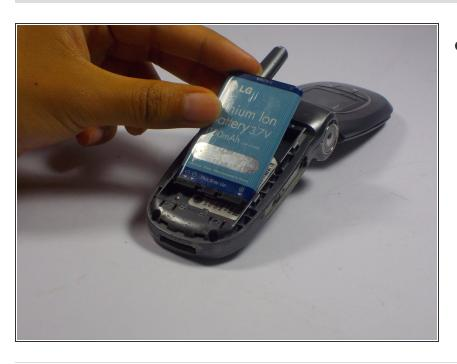
Insert the new Lithium Ion 3.7V 1100mAh battery into the compartment.
