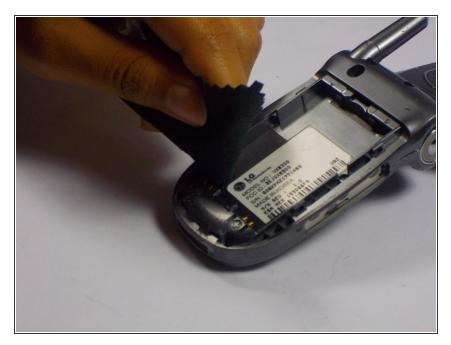
Wipe down the battery compartment to remove any debris or battery acid.
