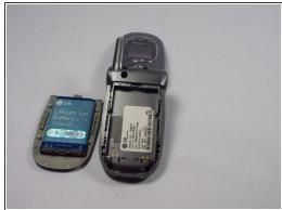
Place your finger into the semicircle gap at the top of the battery, then push down and pull so the battery pops out.
