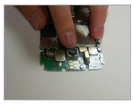
• Remove the rubber cover on the camera by gently lifting it up.
