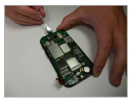
Using the metal spudger, pry the motherboard away from the screen assembly.
