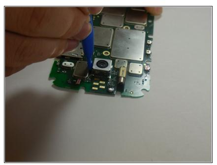
• Use the plastic opening tool to pry the metal housing off.
