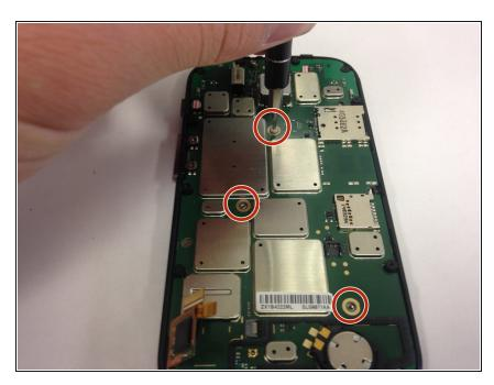
Unscrew the 3- 1mm screws using the T4 torx driver head.
