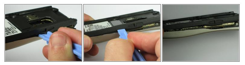
• Insert a plastic opening tool between the faceplate and the black backplate. Gently pry them apart, working from the lower end to the upper side of the phone.
