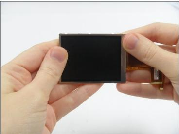
• Slide the LCD Screen out from the Outer Frame.
