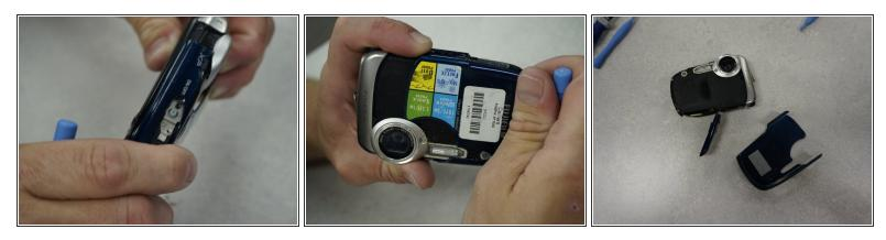
Carefully slide the case to the left. Avoid cracking the case on the lens.
