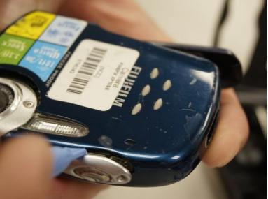
Use a plastic opening tool to detach the case.
