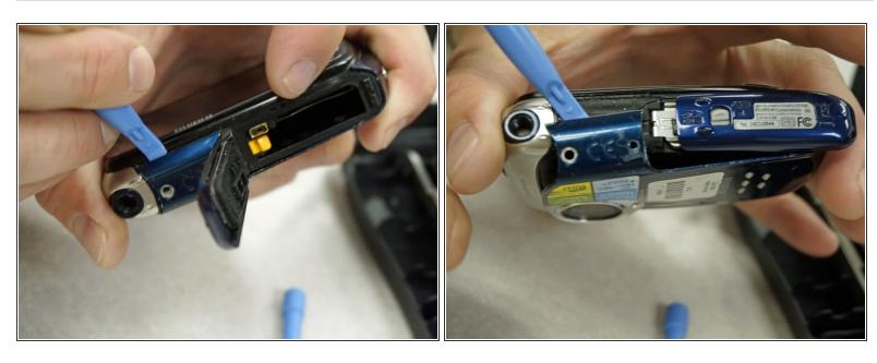
Use the plastic opening tool to cautiously pry the casing off of the camera.
