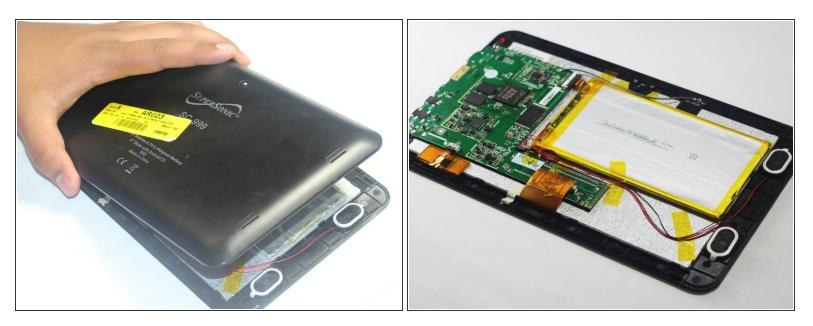
• Lift the back cover from the body of the device to expose the internal components.
