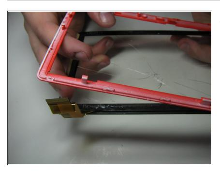
In order to remove the digitizer simply push it out of the casing.
