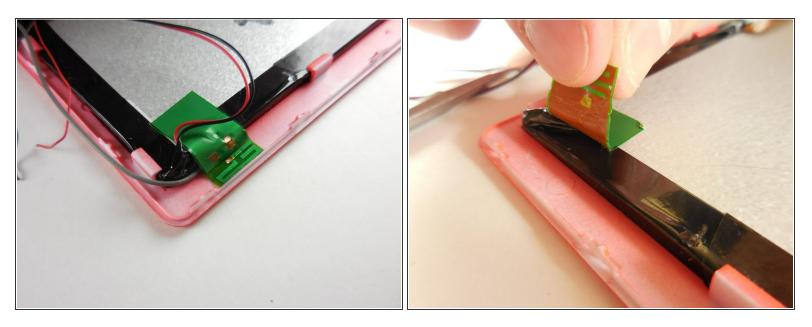
You will see green grounding tape on the bottom left-hand corner of the LCD. Take a spudger and place it between the casing and the tape. Slowly pry up until you can peel the tape back.
