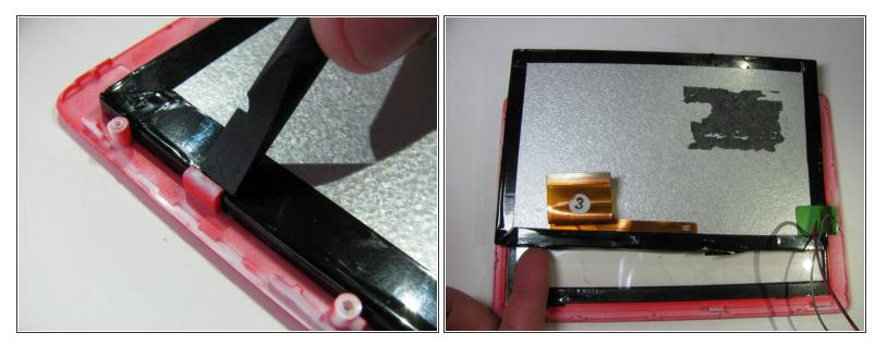
• Remove the LCD from the clips on one side. Pressing sideways, slide the LCD out.
