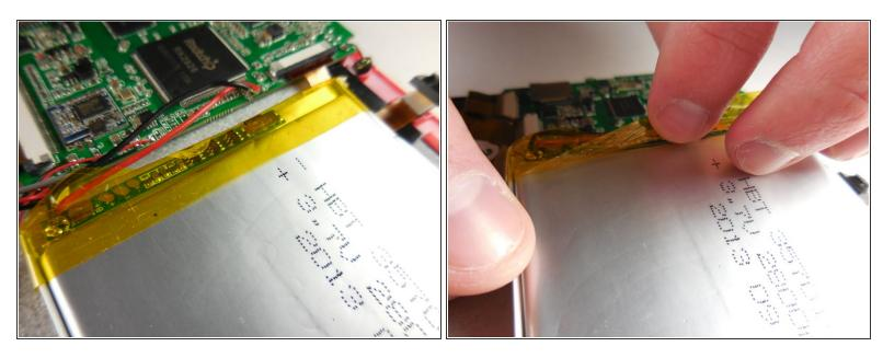
The tape around the battery's circuit board is extremely thorough. There are 2 pieces of tape, on folded over the side and another wrapped around the circuit board. Simply peel both off.
