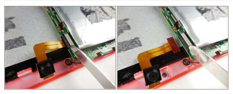
Remove the Camera Ribbon Cable, by holding the clip open and pulling the camera out.
