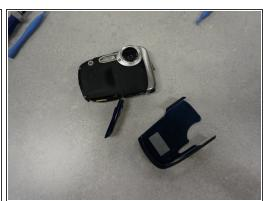
Carefully slide the case to the left. Avoid cracking the case on the lens.
