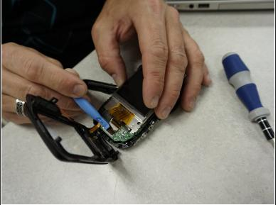
Gently lift up on the black securing bar of the ribbon cable in order to free it from the units motherboard, thus releasing the LCD from the computer.
