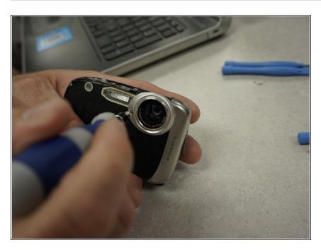
Remove the screws from the lens cover
