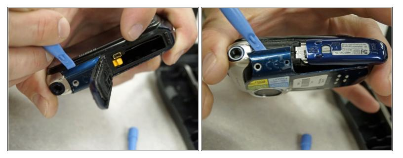
Use the plastic opening tool to cautiously pry the casing off of the camera.
