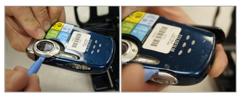
Use a plastic opening tool to detach the case.
