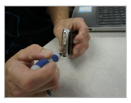
Remove the screws from the side metal cover of outer case.
