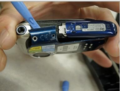
Use the plastic opening tool to cautiously pry the casing off of the camera.
