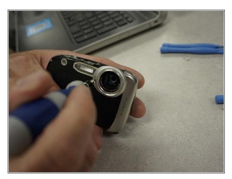
Remove the screws from the lens cover
