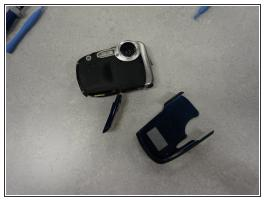
• Carefully slide the case to the left. Avoid cracking the case on the lens.
