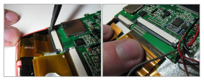
Remove the LCD and Digitizer ribbon cables from the motherboard by holding the clips open and pulling the ribbons out.
