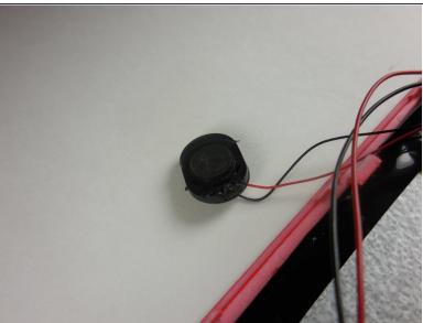
Carefully remove the speaker by inserting the spudger between the case and the speaker. Pry
