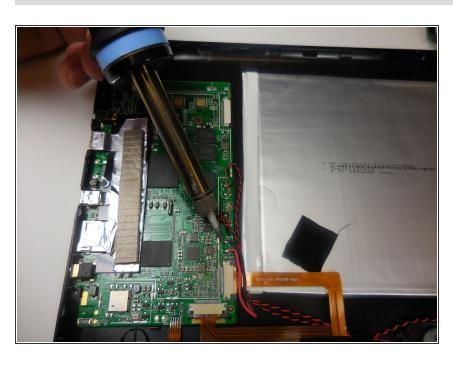
Use a soldering iron to remove the connection between the red wire first then proceed to the black wire.
