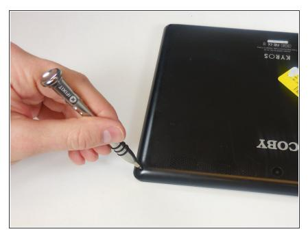
Place the PH00 screwdriver and use it to remove the four 0.5 cm screws from each corner of the tablet.
