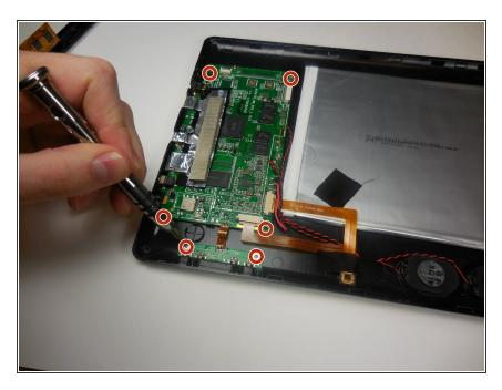
Use the PH00 screwdriver to remove the six 0.25 cm screws circled in the image.
