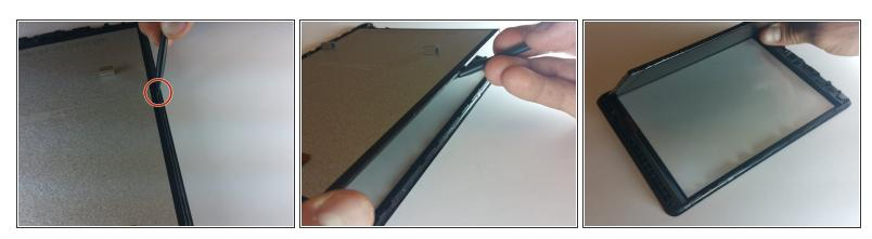
• With the device face down, use a spudger to lift the screen off of the glass from the right side.
