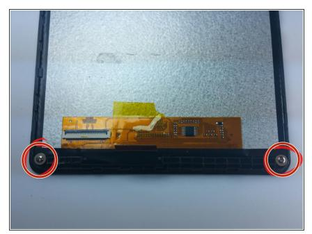
Remove the two silver screws from the bottom of the device.
