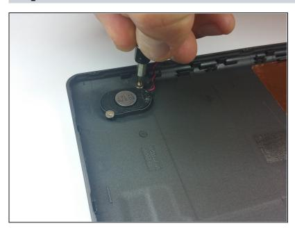
Remove the two 0.116 inch screws holding the speaker assembly in place.
