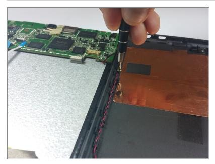
Use a small Phillips screwdriver to remove the 0.116 inch screw holding the red and black wires in place on the inside of the back cover.
