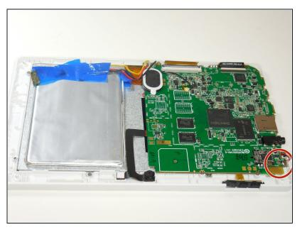
Once the back is off, position the tablet as shown and be sure to warm your soldering iron.
