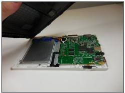
• Use your fingers to pry the rest of the back off; slowly apply pressure from each side to break each clip connection.
