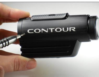
Using the phillips head screwdriver (PH000) remove the two 4.46mm (.175in) screws on each side near the back of the camera.
