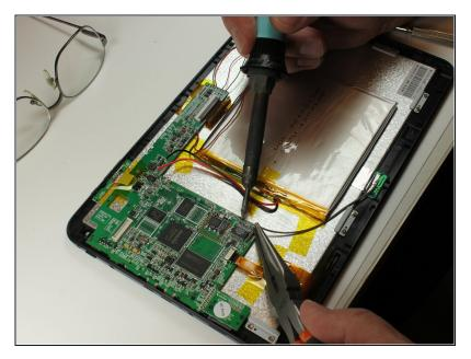
• Solder the outer wire braid shield to the ground point.
