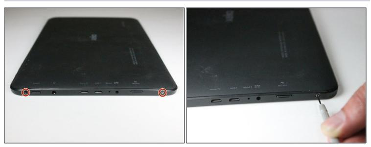
• Remove the two 3 mm retaining screws from the side of the tablet with a Phillips #0 screwdriver.
