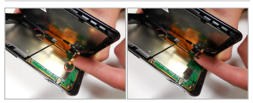
• Pull up on the smaller orange tab with your finger from the circuit board.
