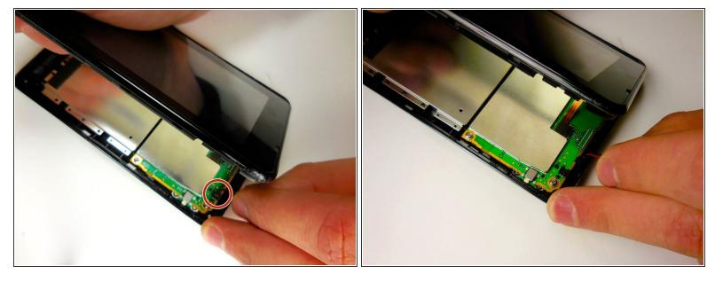
Locate the red and black wire connected to the circuit board with the round, black, rubbery disc
