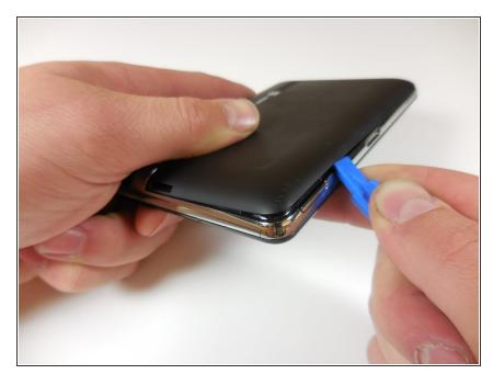
Use the plastic opening tool to separate the tabs on the black back cover of the device by leveraging the tool against the frame around the perimeter of the device.
