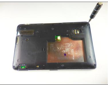
Using the T5 bit, unscrew the four 5.7mm screws in the four corners of the device.
