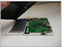
Pry the rest of the back off; slowly apply pressure from each side to break each clip connection.
