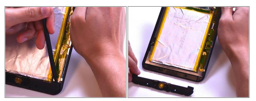
Use the spudger tool to remove the speaker panel carefully.
