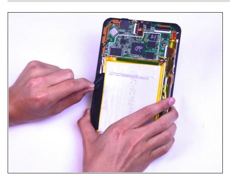
Remove the black tape located to the left of the device.
