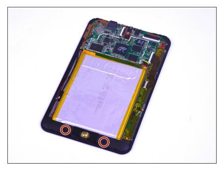
Use a Phillips head #00 screwdriver to remove the two 4.43mm screws on the bottom that keep the speakers in place.
