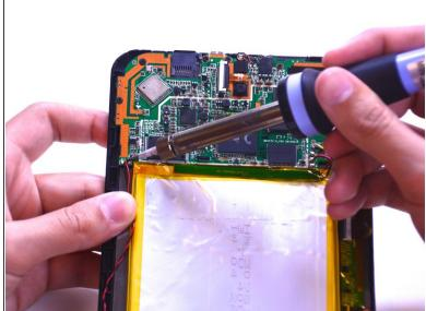
Unsolder the red and black wires connecting the speaker to the motherboard. Take a look at this guide to learn how to solder and unsolder connections.
