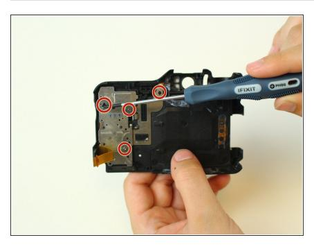
Remove the four screws from the metal plate using a Phillips-head 00 screwdriver.
