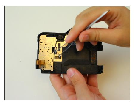
Remove the spring from its socket using precision tweezers allowing the metal plate with the function dial to be removed.
