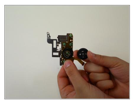
Using precision tweezers, pry the old function dial out of its socket leaving only a black, metal ring attached.
