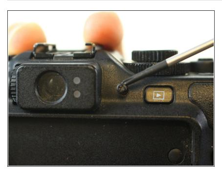
Remove the screw on the right side of the view finder on the back side of the camera.
