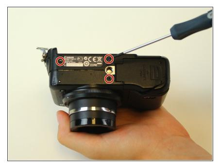
Remove the three screws on the bottom of the camera using a Phillips-head 00 screwdriver.
