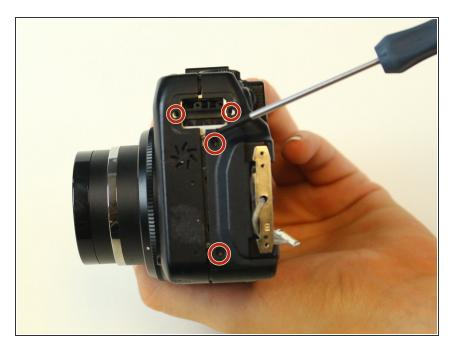
Remove all of the screws on both the left and right side of the camera.
