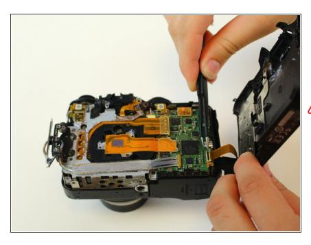
The back case is still attached to the camera with a yellow ribbon cable. The socket has a black flip-up lid that must be flipped up before the cable can be removed. Use precision tweezers to remove the cable.
