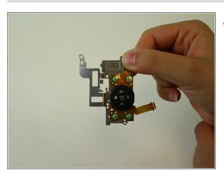
Attach the new function dial simply by pressing it into the black, metal ring until you hear a click.
