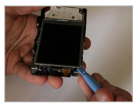
Pop the LCD display out of its frame using the plastic opening tool in order to get to the screws under the
