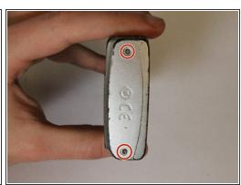
Remove the 6 Phillips #00 exterior screws from the camera. Two are located on the bottom and two are located on either side as shown. Notice that one of the screws is under the AV Out Digital flap on the side. All exterior screws should be 2.4mm in length
