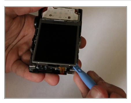
Lift LCD Display using the plastic opening tool to access the screws.
