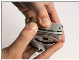
Pry apart the camera casing using the plastic opening tool tool provided. Once the casing has begun to separate pull the two sides apart with your hands.
