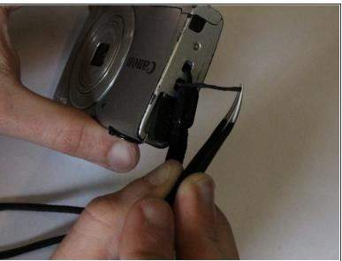
Remove the knot holding the wrist lanyard onto the camera
