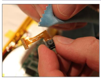
With a <u>microfiber</u> lens cleaning cloth, clean the camera lens
