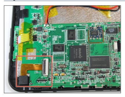
• Locate ribbon connector, make sure it is secure.
