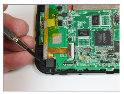
With a plastic opening tool, gently pry the camera body from its retaining socket
