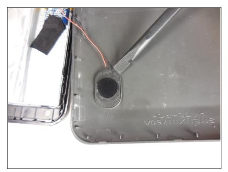
Wedge plastic spudger in between the back panel and the speaker of the device.
