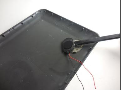
Gently pry out the speaker from the back panel using the plastic spudger.
