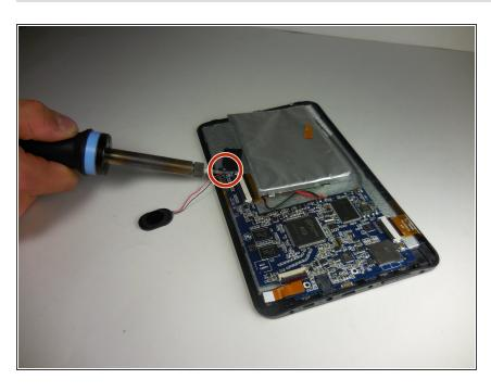
Take the speaker and wires that are attached out of the device and insert a new speaker by soldering the wires to the motherboard.
