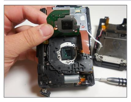
• Lift the metal sheet up to locate the reflective mirror, but do not bend or remove it.
