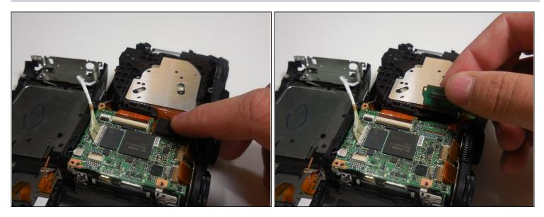
• Lift and detach connector from board as shown.
