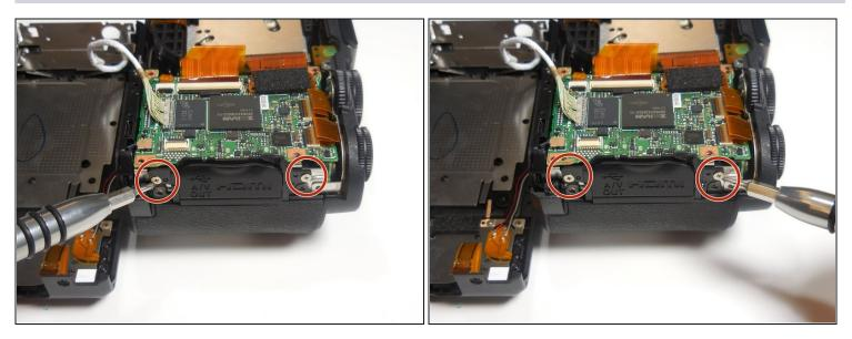
• Remove the two 4.3 mm silver screws on the far right side of the camera using the Phillips #00 screwdriver.
