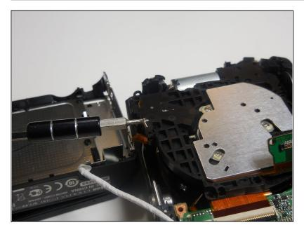
• Remove the board from the camera to locate lens opening
