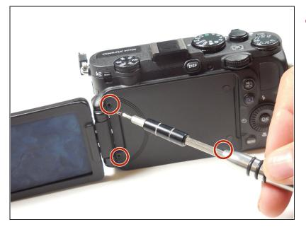
• Open the touch screen, and remove the three 4.3 mm black screws inside using the Phillips #00 screwdriver.
