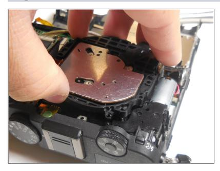
• Lift the metal sheet up and out of the camera.
