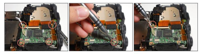
• Remove the four 4.3 mm silver screws located on the ends of the chip using the Phillips #00 screwdriver.
