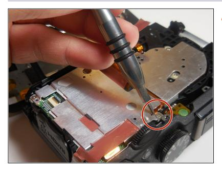
• Once the back casing is off, locate the 4.3 mm silver screw near the top of the camera and remove it using the Phillips #00 screwdriver.
