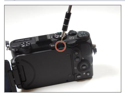
• Remove the 4.3 mm black screw on top of the camera, right above where the screen folds out. Use the Phillips #00 screwdriver.
