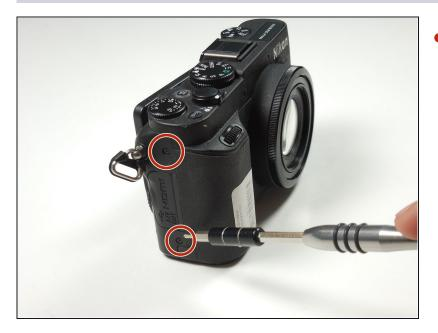
• Remove the two 4.3 mm black screws on the right side of the camera using the Phillips #00 screwdriver.
