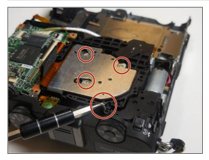
• Remove the 4.3 mm screws from the metal sheet using the Phillips #00 screwdriver.
