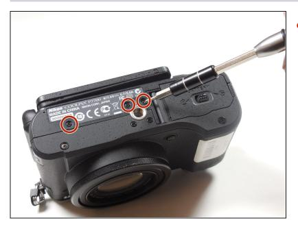
• Remove the 4.3 mm black screws on the bottom of the camera using the Phillips #00 screwdriver.
