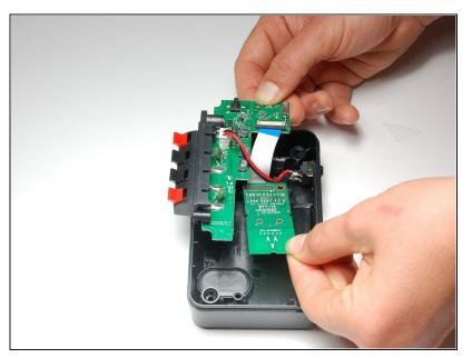
• Flip over the motherboard and wireless audio module chip.
