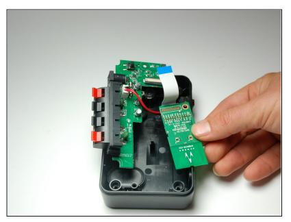
Using your fingers, pull the ribbon wire out from the black retaining flap in order to completely disconnect the wireless audio module chip.
