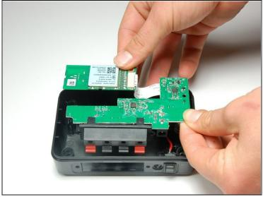
• Using both thumbs, push the front speaker input terminal back towards the inside part of the device.
