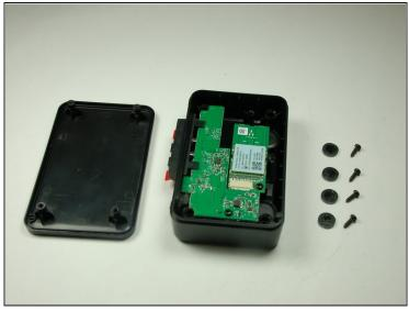
• Flip the device over and remove the top casing from the sender.
